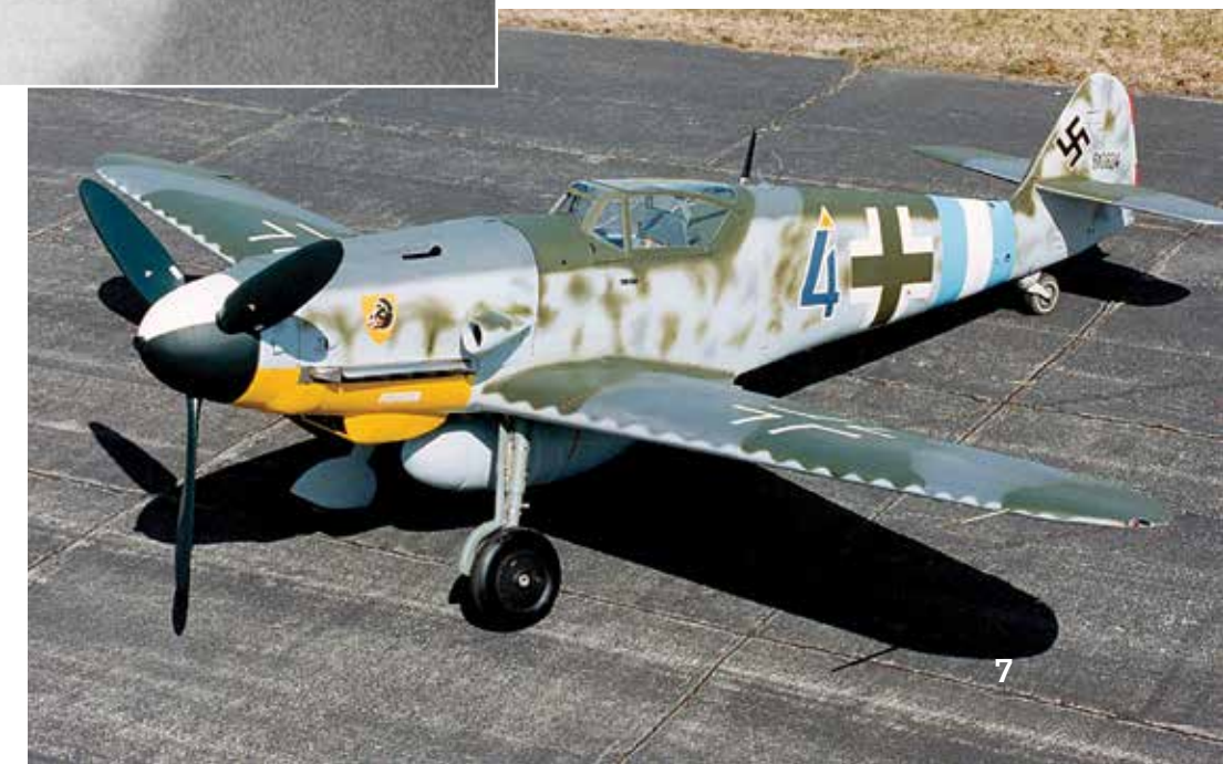
Below: Later models of the Messerschmitt Bf 109s concentrated their firepower in the nose, with guns firing above and through the centre of the engine.
