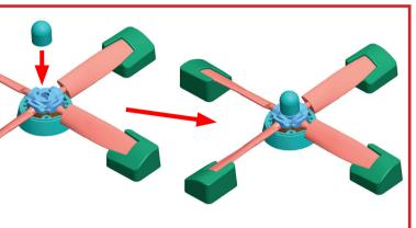
Place the dom shell **01H** carefully onto the three pins of the completed hub and fix it using glue.
