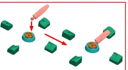
Take one of the four propeller blades **01F** and insert its tip inside the block to ensure the correct angle. The pinion will fit comfortably onto the crown if the angle is as shown in this diagram.
