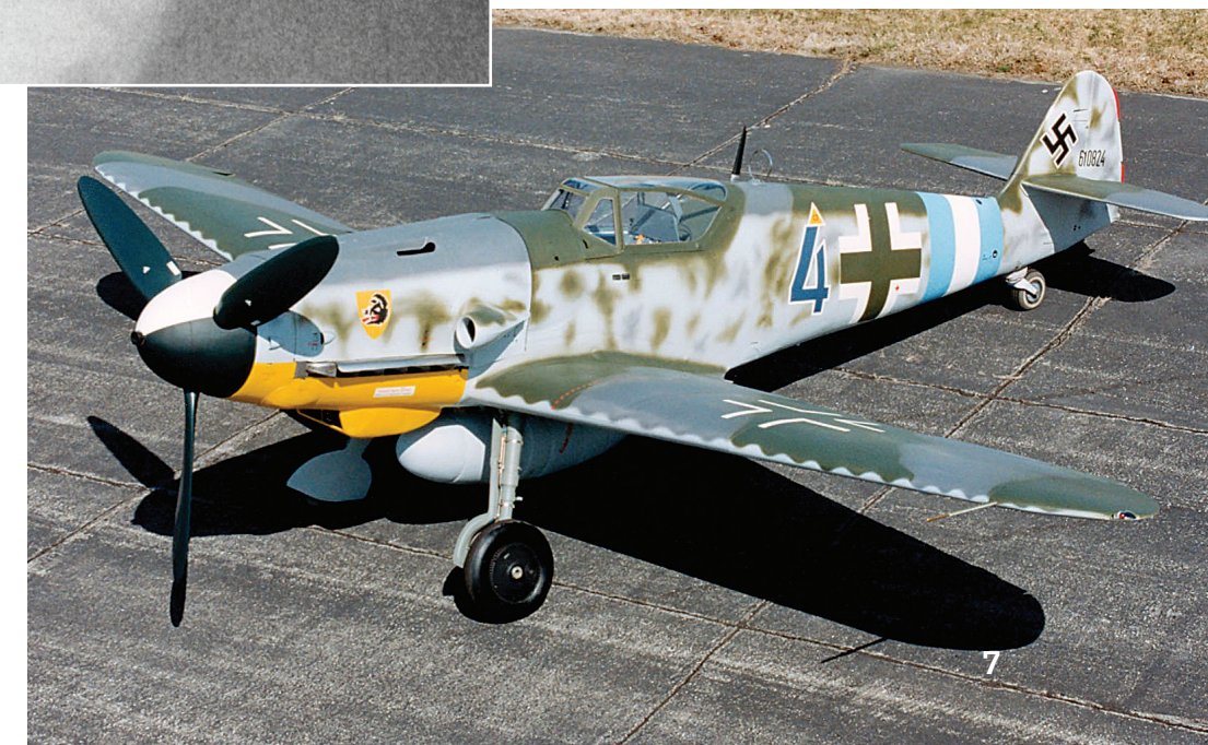
Below: Later models of the Messerschmitt Bf 109s concentrated their firepower in the nose, with guns firing above and through the centre of the engine.
